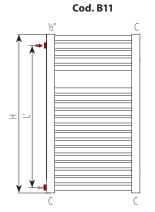
Couplings welded laterally in alignment with the first and the last element on the left side
