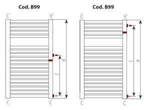
Lateral connections at connection centre personalized (2 manifolds + diaphragm)
