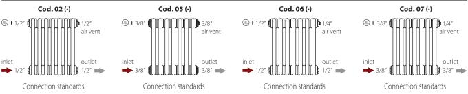
• For TESI radiators lower than 1000 mm or radiators with more than 15 sections.
