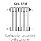
Other configurations are possible with different bush diameters: 1"; 3/4"; 1/2"; 3/8" and 1/4" blind
